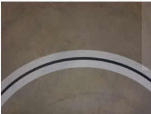
Sticker AGV track curve 90° b=160mm r=1m
